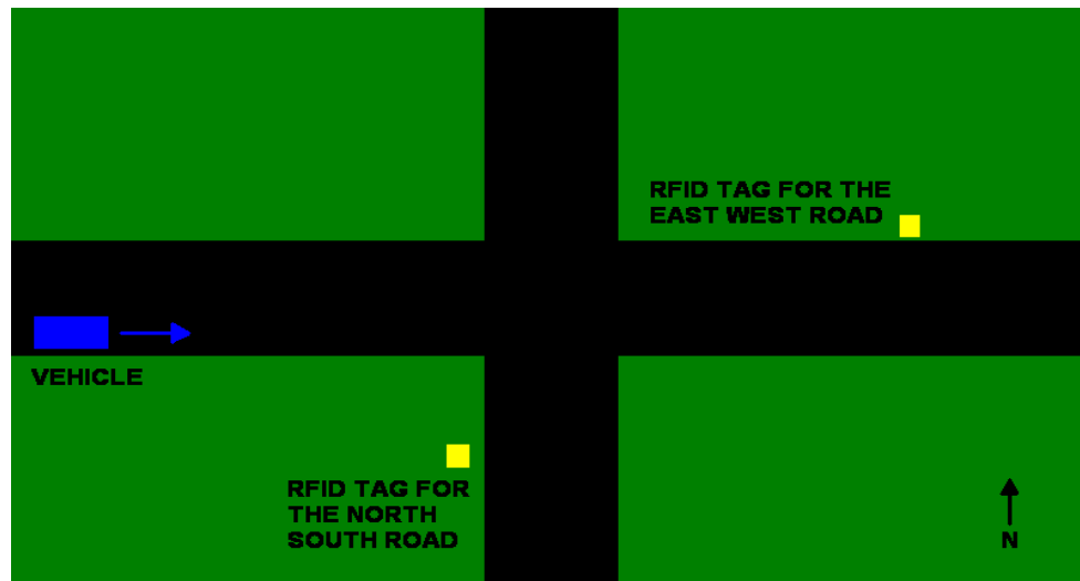
Figure 2: Graphic illustrating the issues of using tag distance to determine which tag to use and why adding cardinal directions to the tags will solve this issue.
