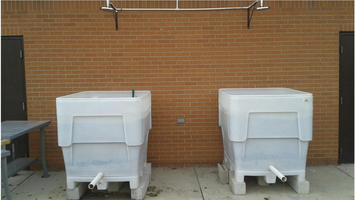
**Figure 2. Rain garden test cells and shower heads.**
